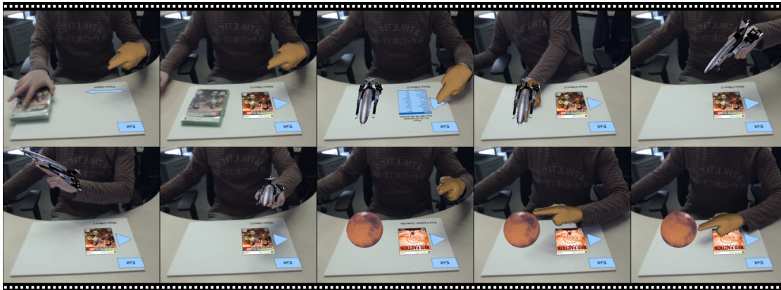
Fig. 10. Example human-computer interface based on our tracker – the user places a DVD on the surface, prompting the system to show facts about the DVD and a 3D object related to it, which he/she can manipulate with the hand. In the case of the first DVD the user sees and can be pick up and move a 3D model of a starship. In the case of the second DVD, the user sees and can rotate a model of planet Mars.
