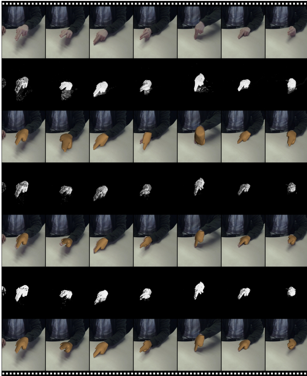
Fig. 7. Filmstrip showing the per pixel difference between the foreground and background probabilities P_f - P_b , where P_f - P_b > 0 , and the resulting recovered pose, when using fixed bin size histograms (rows 2 and 3), variable bin size histograms (rows 4 and 5) and variable bin size histogram combined with temporal consistency (rows 6 and 7).
